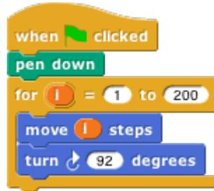
The input to the **move** block is an orange oval. To get it there, drag the orange oval that's part of the **for** block:
